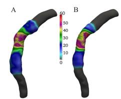
Figure 4: Distribution of the force that causes the deformation of the arterial wall; A – simulation using the simplified numerical model; B –simulation using the hyperelastic numerical model; units on the scale bar are in mN
