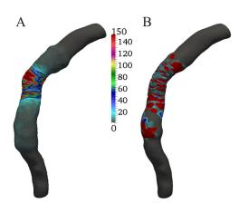
Figure 5: Distribution of the von-Mises stress, calculated based on the deformation of the arterial wall; A – simulation using the simplified numerical model; B –simulation using the hyperelastic numerical model; units on the scale bar are in kPa
